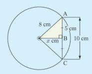
The shortest distance is the 'perpendicular distance'. The line drawn from the centre of a circle, at right angles to a chord, bisects the chord, so
